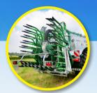
Compact, double folding system at the back of the tanker
